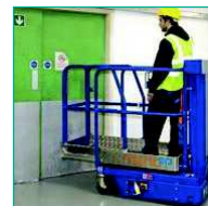
Passenger lift 4.50 m high
